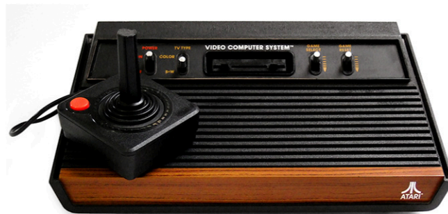
FIGURE 15.17 The Atari Video Computer System, 1977. Released in 1977, the Atari Video Computer System could be connected to almost any television, allowing users to play video games at home. The software was stored on small plastic cartridges that were plugged directly into the machine. (credit: “Atari 2600 mit Joystick” by “joho345”/Wikimedia Commons, Public Domain)
