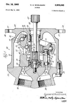
Figure 1.14 USPTO Patent No. 2956845 for an axial piston pump. (credit: modification of work by Gunnar A. Wahlmark, Rockford, Illinois USA. via Wikimedia Commons / Public domain)
