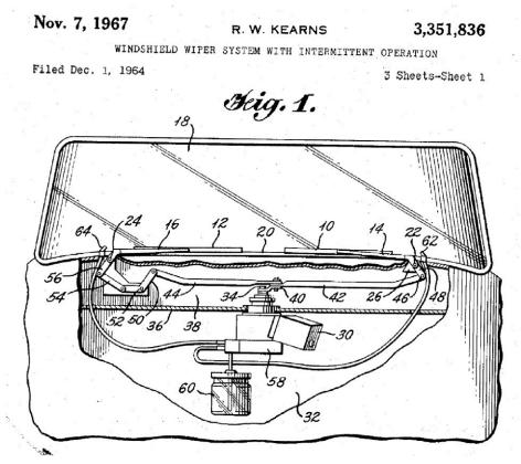
Figure 2.4 Patent for windshield wiper system with intermittent operation. (credit: USPTO doc ID 03351836 / )
