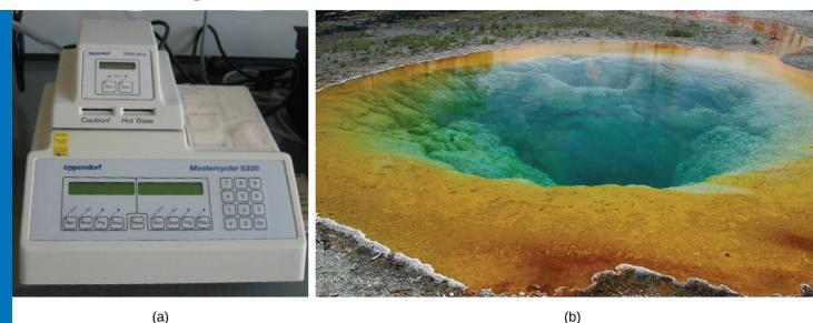
FIGURE 10.1 (a) A thermal cycler, such as the one shown here, is a basic tool used to study DNA in a process called the polymerase chain reaction (PCR). The polymerase enzyme most often used with PCR comes from a strain of bacteria that lives in (b) the hot springs of Yellowstone National Park. (credit a: modification of work by Magnus Manske; credit b: modification of work by Jon Sullivan)
