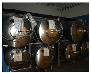
FIGURE 4.18 Fermentation of grape juice to make wine produces CO<sub>2</sub> as a byproduct. Fermentation tanks have valves so that pressure inside the tanks can be released.
